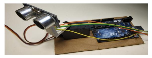
Now, we have to connect sonar sensor to arduino. Be careful while connecting VCC and GND of the sensor to 5v and GND of arduino respectively. Later, connect the trig pin to 8 and echo pin to 9 of arduino.
