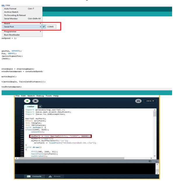
Now, we have to find the COM Port number. Go to Arduino IDE and find the Com port(COM3 in photo). Put the COM port number in line 13 of processing code (COM3 in photo).
