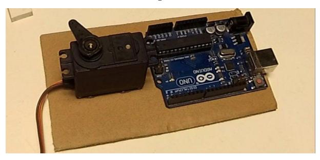
First of all, we have to cut a card board (15cm \* 8cm). Then, glue arduino and servo motor on it.
