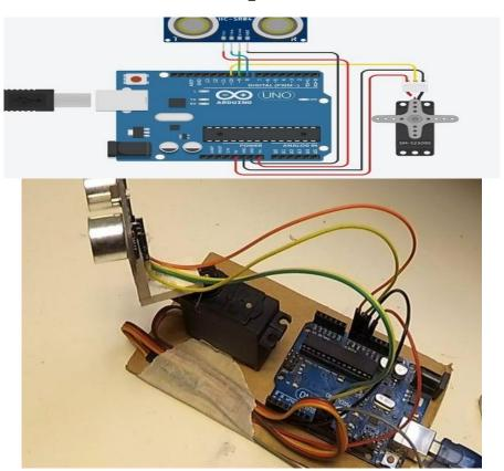
After connecting sensor to arduino it's time to attach servo motor with it. Again, be cautious about connecting VCC and GND of servomotor. Connect servo signal to pin 10 of arduino.
