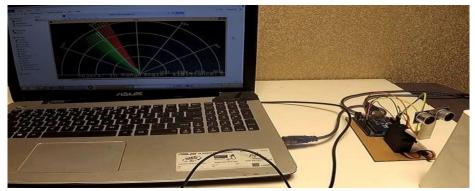
Finally, pressing the Run button will show a processing window. It will show both servo angle of the radar and the object distance.
