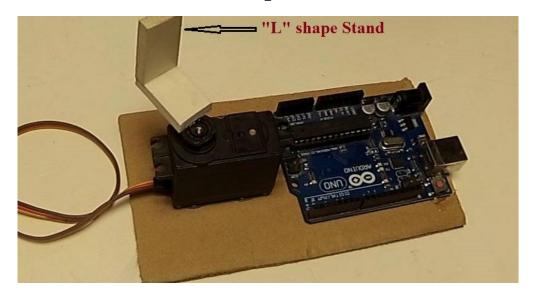
Now, we have to make a "L" shape stand for Ultrasonic sensor (HC-SR04) which keeps it still on the servo motor.
